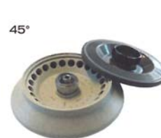
Angle rotor, 24-place, Cat. No. 01226 n= 13,300 min -1 , max RCF 17,008
