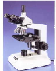
ML2300 trinocular A sliding beam splitter directs 100% of the light to the eyepieces or 80% to the camera and 20% to the eyepiece
