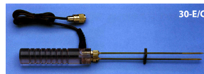
30-E/C Used for bales, 9 1/2" insulated pins, with 8 1/4" penetration, eliminate the effect of surface moisture
